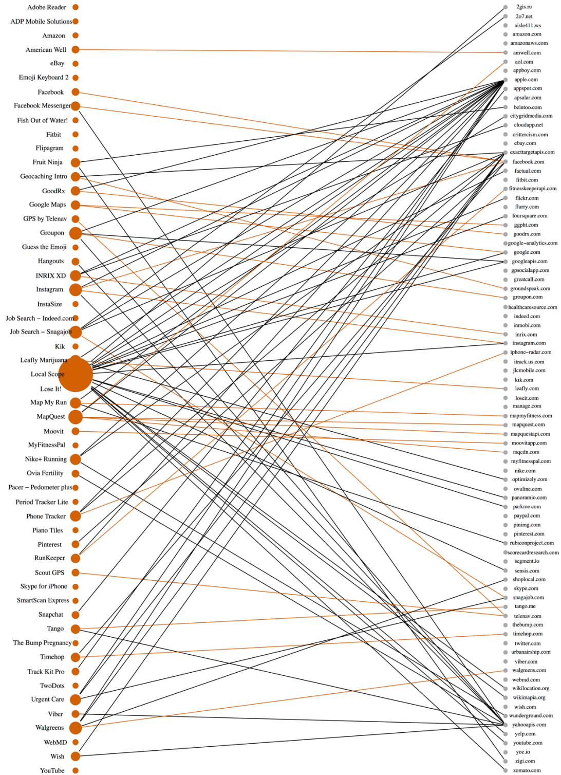
Figure 8. Location data sharing by iOS apps. The color of the line indicates whether the domain is that of the primary maker (orange) of the app or of a third party (black). Apps with bigger circles shared location data with more domains, both primary and third-party.
